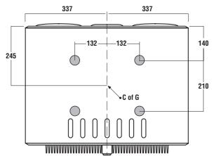
Positioning the feet relative to the C of G
